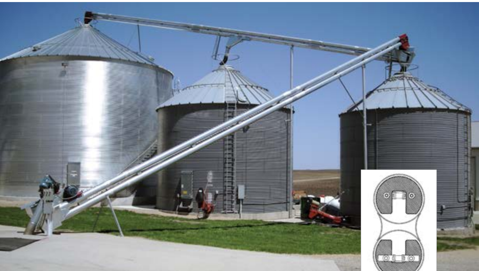
Stationary grain pumps can be used in various applications at angles from horizontal to 60°. Lengths available in 5' increments. A flow through inlet is convenient for overhead applications. Cross section of housing
