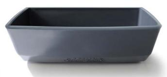
In some cases, YORK will quote the **CC style low profile** bucket which allows for closer bucket spacing on the belt, thus increasing elevator capacity. Low profile buckets have the same characteristics and construction of the standard bucket, varying only in depth and weight. Capacity on this bucket style is based on water level +5%.
