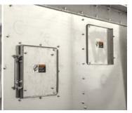
**Lagging inspection door** features hinges and quick latch for convenience.
