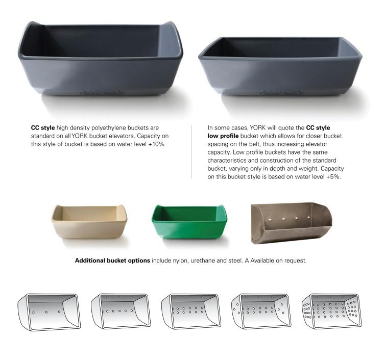
Vented buckets improve bucket fill and discharge when moving lightweight, fluffy materials or materials that are extremely dense or flow poorly at high speeds. These materials may include various flours, meals, feed mash or screenings. The vents remove trapped air and improve bucket efficiency. Vented buckets are available on request.
