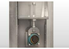
**3-7/16" (87 mm) heavy-duty ball bearings** and heavy-duty take-up assembly for powerful performance under rugged conditions.
