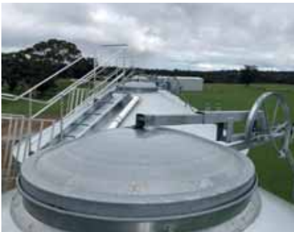
Inlet: Easy to operate, Bird's ground operated lid has a unique action and is one of the better designed lids inspected.
