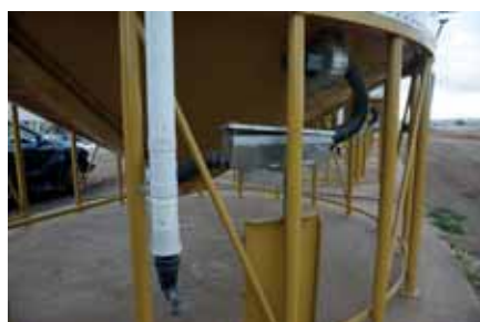
Fumigation: Ground-application of phosphine unitises one of the aeration fans plumbed via the phosphine box.
