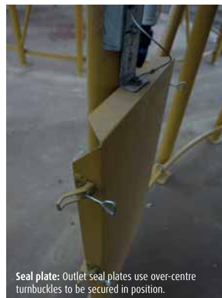
Laser cut and folded over-centre latches as used by a number of other manufacturers including Denny's silos, seem a little lightly constructed.
