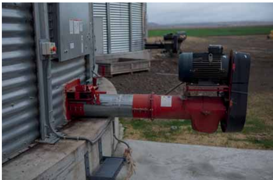
Outlet: The outloading auger door actuators were simple to operate.
