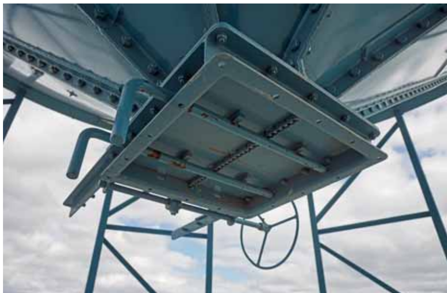
Slider: The outlet slide gate uses a wheel and geared axle to open and close the outlet gate. This gate becomes the sealing plate with two eccentric pins rotate to push the plate up to seal the outlet.
