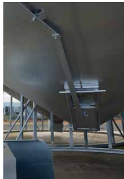
Outlet: A slide gate operable standing outside the base is simple to use.
