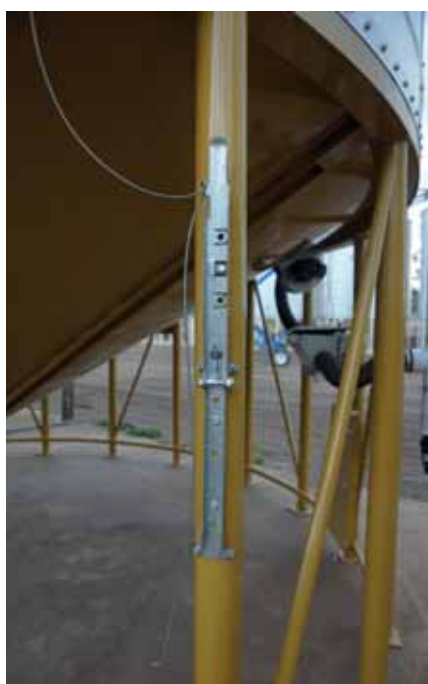
Laser cut and folded over-centre latches as used by a number of other manufacturers including Denny's silos, seem a little lightly constructed.
