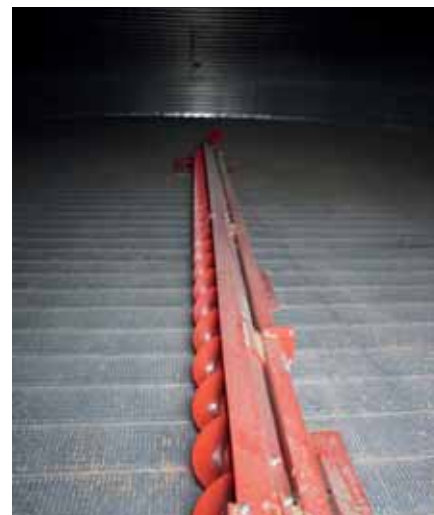
Inside: Twister silos have full floor aeration and a sweep auger.
