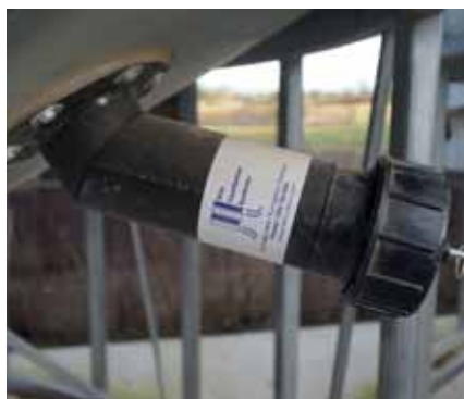
Fumigation: Phosphine ground application systems are mounted to the cone but would benefit with connection to the headspace.
