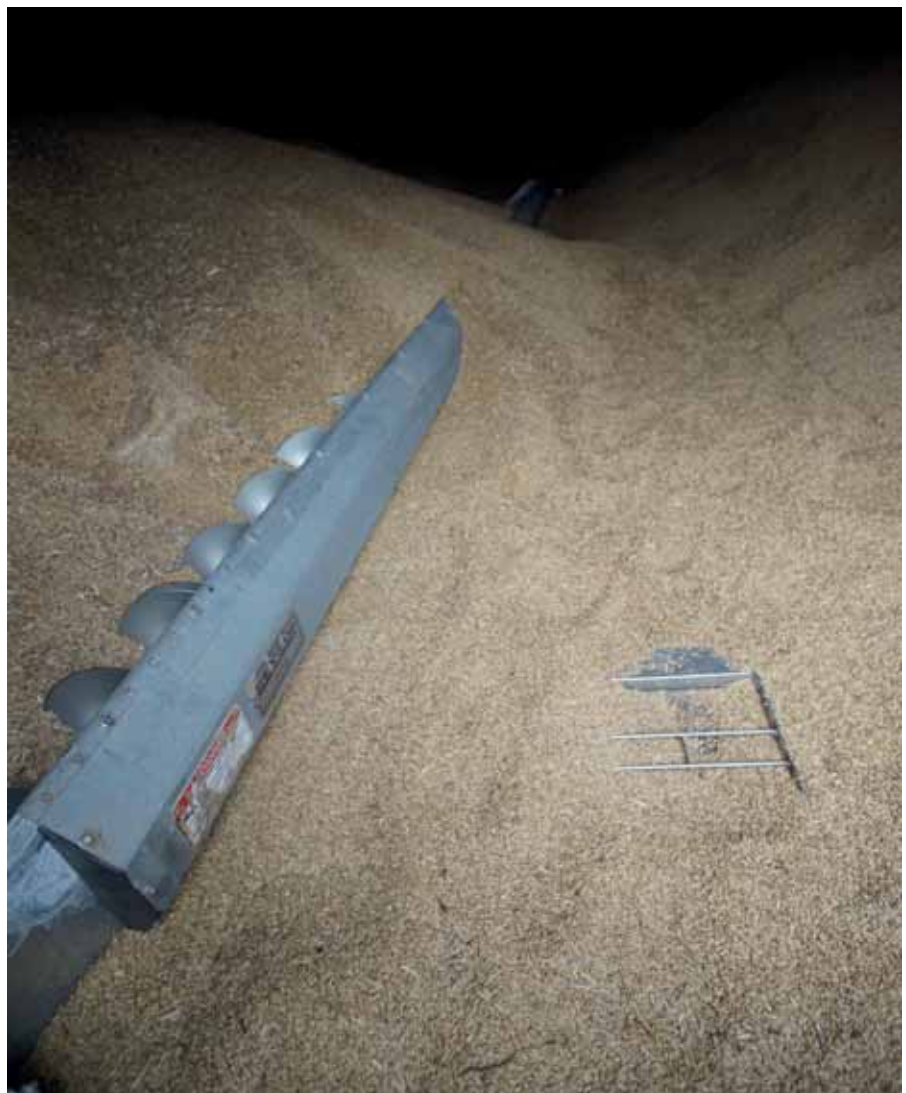
Clean sweep: A good sweep auger will remove almost all of the grain in the silo minimising the volume that has to be swept up.
