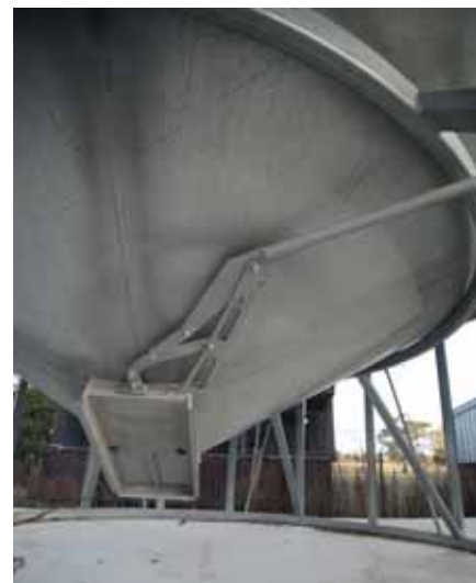
Outlet: Clever geometry and laser-cut profile components actuate the outlet slide but the operator has to crawl into the silo base frame to operate it.
