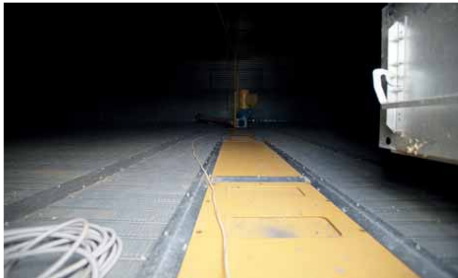
Full-floor aeration provides uniform air flow but must be pulled up to fully clean out.
